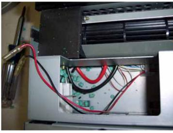
This picture shows where 9 wires were gnawed or cut in half. The mice must have been hungry!
