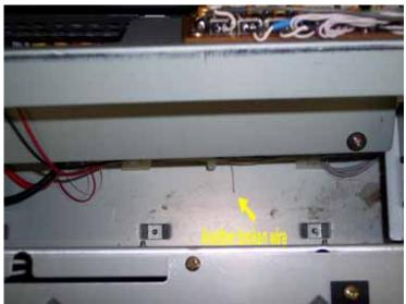
I Fixed this broken wire and of course I again had +13 V at the appropriate pin on J4005, the 1st LO worked again, and the FT 1000 MP was restored to its previous excellent working condition.
